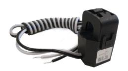
**TRA1 80A transformers** are current transformers specially designed for being installed at the top of a circuit breaker. All the models have secondary of 250 mA and are suitable for SEM One, SEM Three and third-party devices.
