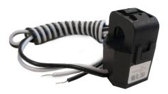
**TRA1 250A transformers** are current transformers specially designed for being installed at the top of a circuit breaker. All the models have secondary of 250 mA and are suitable for SEM One, SEM Three and third-party devices.
